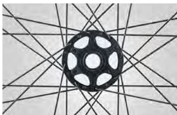
32 crossed spokes pattern, with stainless steel spokes and brass nipples.
