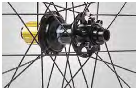
Specially designed and developed e-bike hubs, with oversized rear hub ratchet and ring to withstand powers up to 550 Nm. Available 110mm/148mm Boost O.L.D. for IS6 standard disc rotors mounting. Assembled with high-smoothness bearings.
