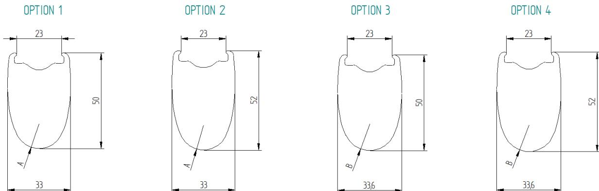
The four variants formed the initial core of the study to identify the profile with the greatest potential in terms of aerodynamic efficiency, stability, and airflow continuity between tyre and rim.
