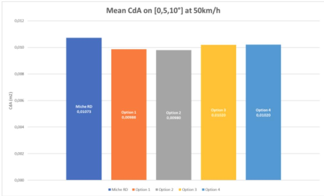
Preliminary results from the CFD analysis indicate that all designs improved over the Kleos RD 50 rim, with option 2 having the lowest Cd·A, for which an improvement of 8.6% at 50 km/h is expected.
