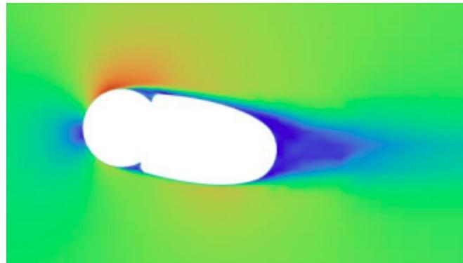
This result was made possible by improved integration between the tire and the rim, which, combined with the rim's NACA profile, ensures better airflow attachment even at high flow incidence angles, thereby leading to an overall reduction in drag.
